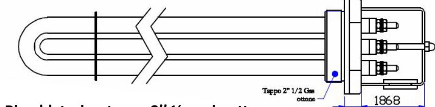
**Custodia in alluminio 100x100 mm.**
